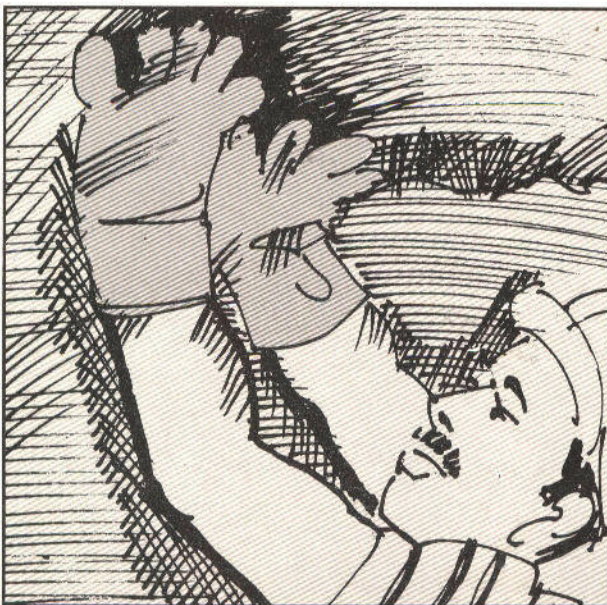
AQUA PLUG held in place to completely stop flow of water
